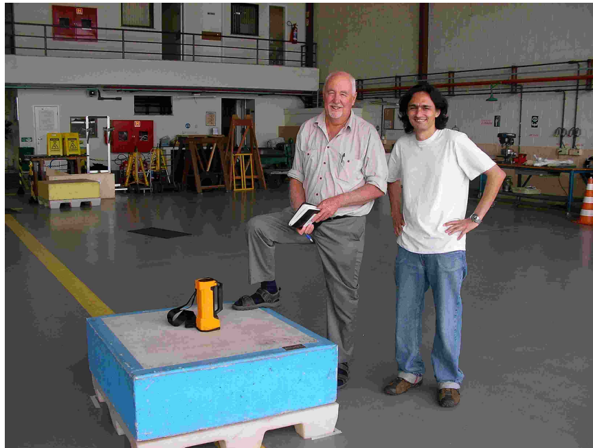
Figure 1. Calibrating the RS-230 gamma ray spectrometer on the Fugro pads.
